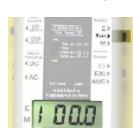
Set the switch "field type" to the "Test" position. On the left-hand side of the display a "1" will appear, and on the right-hand side either "00.0" or "000", depending on the selected measurement range. A higher measurement value reflects the current additional tolerance of the instrument.
