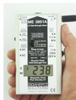
Insert the plug of the enclosed grounding cable into the dedicated socket of the meter and run the cable along the side of the case to the back (see picture). Make sure that neither the grounding cable nor the user’s hand is in the front of the meter (falsifies the reading!).
