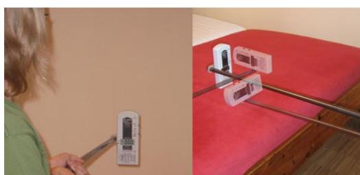
Some guidelines recommend the so-called “potential-free” measurement of electric fields, i.e. without needing to ground the meter. A potential-free measurement is, in principle, very adequate for the
