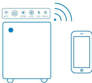
The air purifier can also be automatically regulated based on the air quality readings from the built-in sensors (280i), or the optional external air quality monitor Blueair Aware™ (205)
