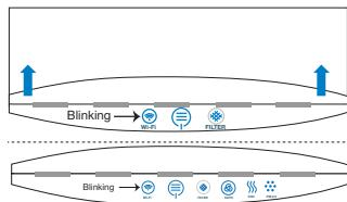
Open the flip-up lid and press the airflow speed touch button. When the Wi-Fi symbol starts to blink, the air purifier can be paired with the Blueair Friend mobile app.
